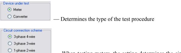
— When testing meters, the setting determines the circuit connection of the meter under test
